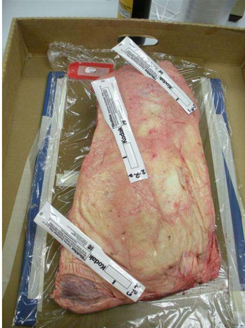
Alanine dosimeters placed on the surface of each cut
