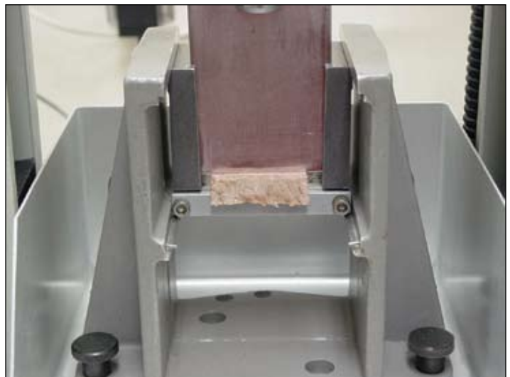
Slice shearing on a universal testing machine
