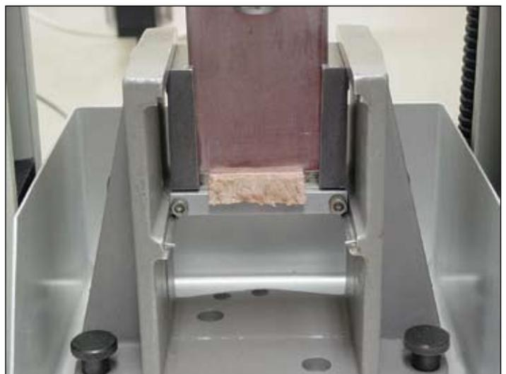
Slice shearing on a universal testing machine
