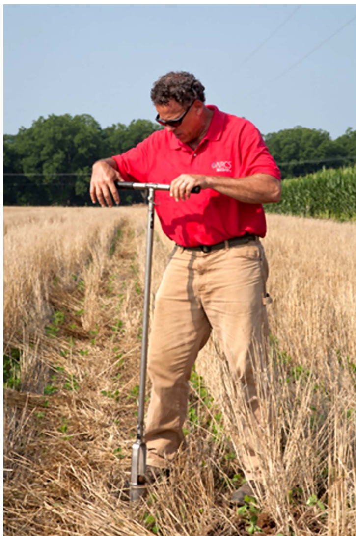
Figure 2. A National Resources Conservation Service (USDA-NRCS) employee collects a soil sample in Virginia. Eighty-three percent of beef producers who responded to the survey sampled their soil at least once every 4 years. Soil nutrient analysis is a key component of nutrient management planning and necessary for applying manure and synthetic fertilizers at agronomic rates (amounts the plants need, while minimizing risks of nutrient leaching and runoff).
