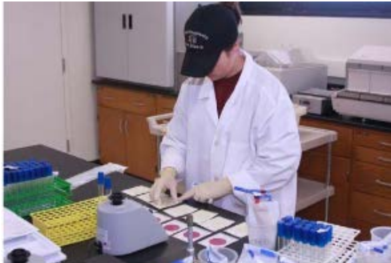
Figure 3. Using a spreader to distribute the inoculum in the circular area of the APC and E. coli and Coliform Petrifilm plates.
