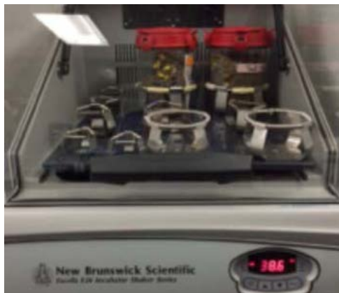
Figure 2. Simulation of the cow digestive system with an anaerobic atmosphere, typical cow body temperature and slight shaking to mimic peristaltic motion.
