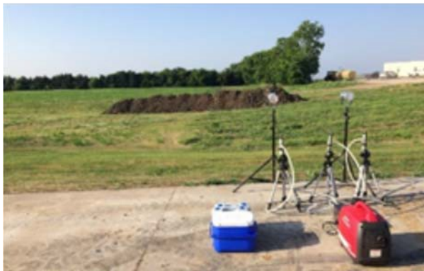
Image 1. Impinger and impactor systems placed approximately 50m downwind from the manure stockpile from cattle fed with chlortetracycline for bioaerosol collection.
