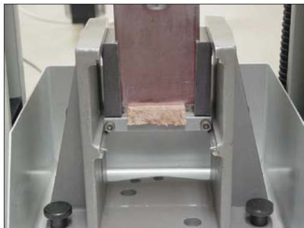
Slice shearing on a universal testing machine
